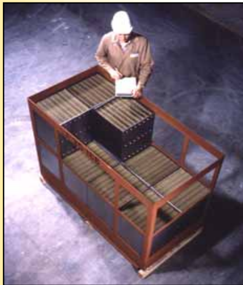
Catalyst elements being loaded into a frame
